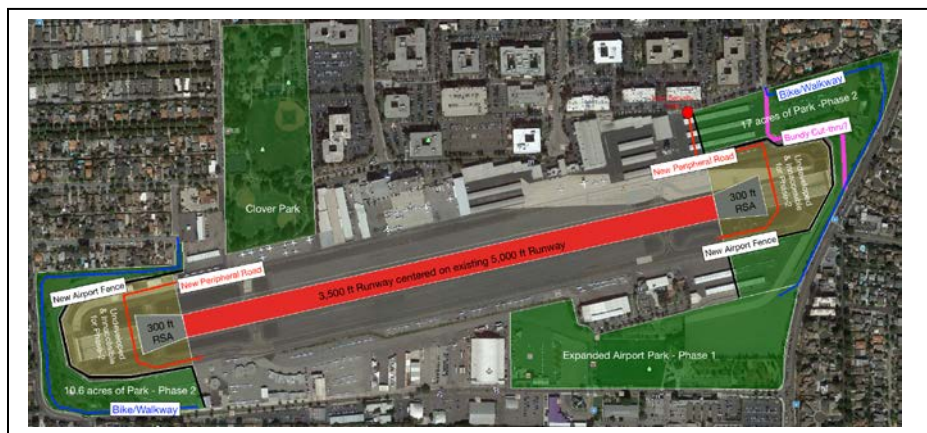
Plans for shortening the Santa Monica Airport runway from 4,973 to 3,500 feet in length
